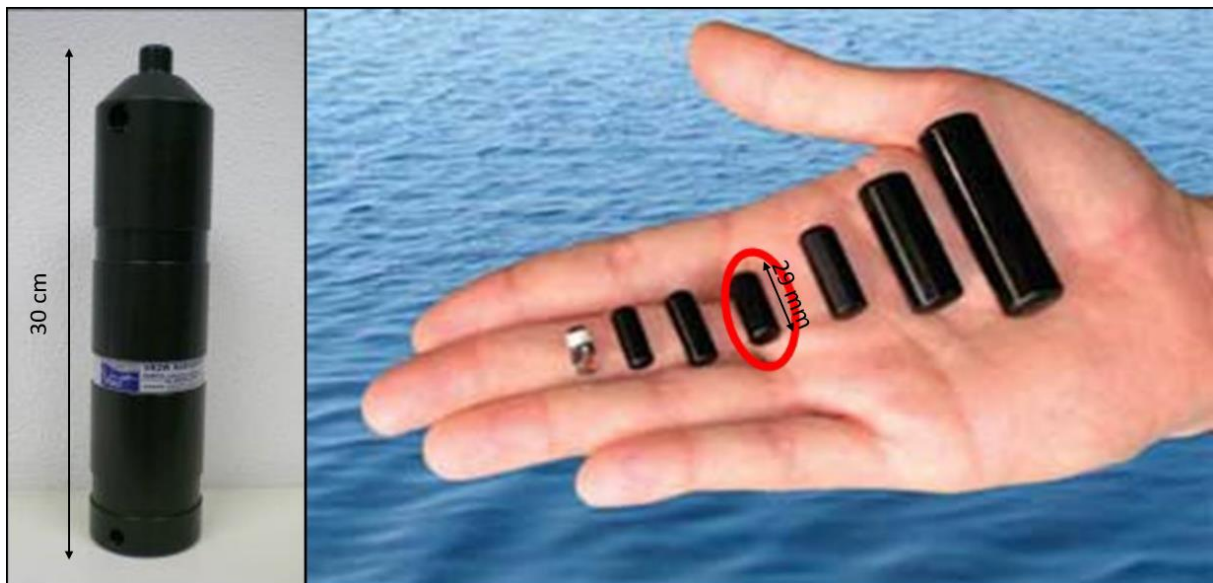
Figure 4: Vemco VR2W receiver (left) and Vemco V9-2L (circled) acoustic transmitter (right) (Winter et al., 2018)
