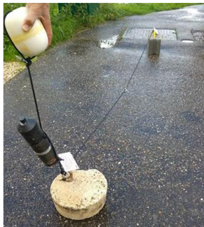
Figure 5: Vemco VR2W receiver with two weights and one floater on a short rope (Winter et al., 2018)
